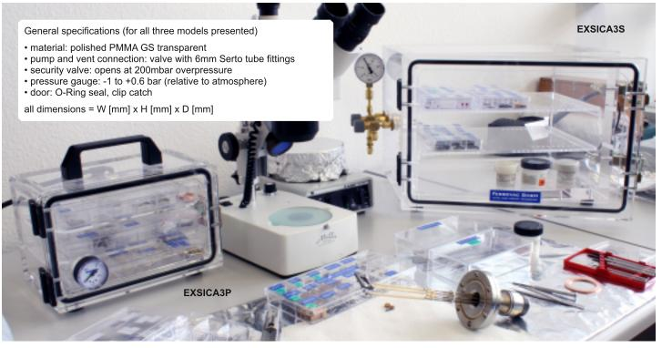
After pumpdown with a membrane pump, the exsiccator holds a base pressure of approximately 25mbar (absolute) over a period of several months. A pressure meter roughly indicates the vacuum level. The box can be filled with dry Nitrogen or Argon if desired. An overpressure valve is provided for safety reasons. Standard, portable and extrawide versions of the vacuum desiccator are available.
